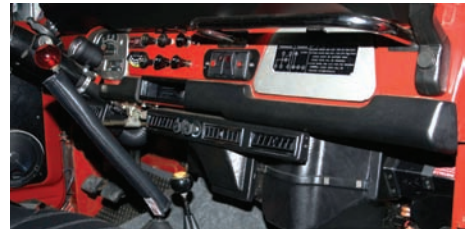
U.S. spec Toyota FJ-40 Land Cruiser dash using factory controls and Vintage Air louvers.
