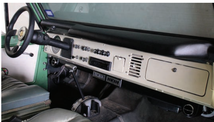
Ford Bronco dash with SureFit system with full width plenum, controls and Vintage Air louvers. 4-vent kit also available.
