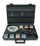
424007 Hydra Crimp Kit. Portable hand held hydraulic crimper. Beadlock A/C Hose Crimper, 134a.
